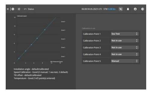
Offset adjustment adjusts any angular mounting variations relative to the ship. The adjustment can be up to +-180 degrees, however some sensors do not have as good resolution at higher adjustment angles so installation should aim to be as close to zero as possible.
