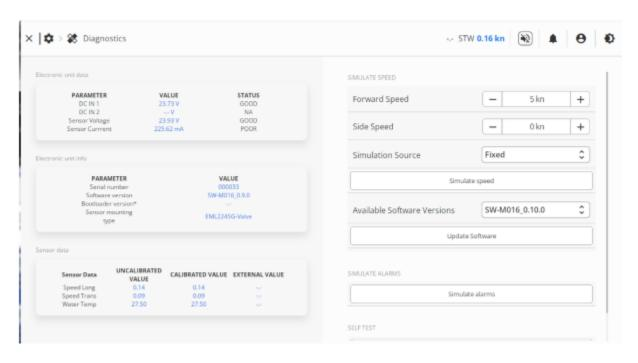
The Diagnostic screen has a number of useful functions to help diagnose problems. If serious problems occur, this can be indicated in the alerts page as caution or warning. The left side of the page shows the running status of the system, showing internal measurements such as voltages and currents with their advised limits.
