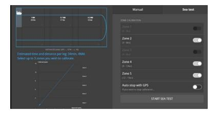
once selected, the vessel should move into position for the start of the leg and accelerate to the correct speed .
