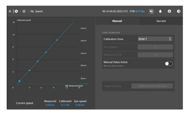
If you wish to adjust an individual speed offset The right side of the screen shows the current values, these are either previously adjusted manual settings, default or generated by the sea test. if not active, these can be adjusted by activating the desired speed zone, and adjusting the real speed (from GPS) and the measured speed from the sensor.
