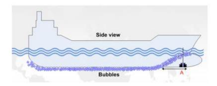
For 2 axis speed logs the transducer should be positioned as deep as possible on the hull. The transmitting surface of the transducer must be installed horizontally.
