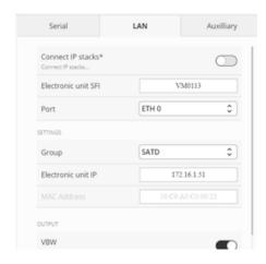
The LAN settings allow System function ID (SFI to be set (the same on both LAN ports), the transmission Group and the IP to be set. The 2 IP addresses cannot be within the same domain defaults are 172.16.1.50 and 172.16.2.51.
