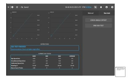
The user can then decide to check the installation angles measured during this sea test. if these seem wrong, they can be ignored and manually adjusted to a more appropriate value
