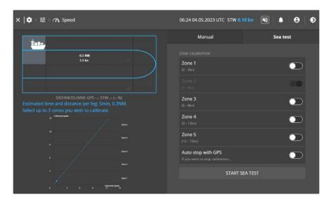
Sea calibrations should be made at max speed and normal operational speeds. Select the desired speed zones to be calibrated, and then follow the onscreen instructions. The calibration should take place in an area with low current or stable current, and the opposing legs should be in the same area, preferably not in the wake of a previous leg.
