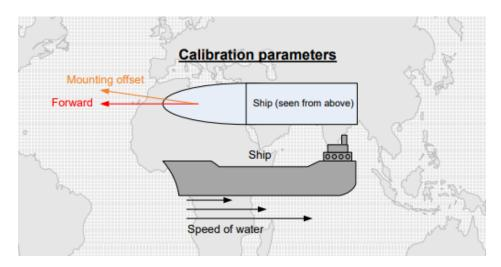
Sensor calibration can vary at different speeds of the vessel due to drag of the water, or bubble / Turbulance formation, so the system has possibility to calibrate the sensor at 5 different speed zones. Each can be adjusted manually, using a sea test of 2 legs, or automatically using inputs from other approved systems.
