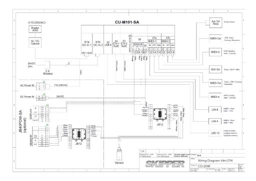
Connection can be direct to the sensor from the sensor port, or via an optional JB40 Electronic buffer unit. The JB40 unit can be mounted near the sensor or on the bridge, and provides a buffer and diagnostic port for the unit.
