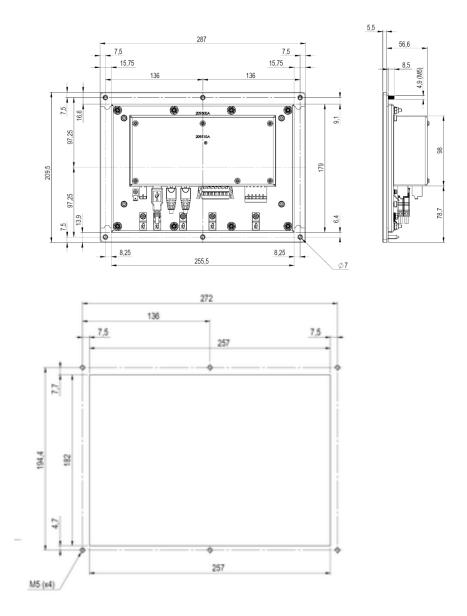
For rear mounting or if IP56 is required the display should be back mounted using CU-IP56 clips (Art number M-KIT-CU-IP56).
