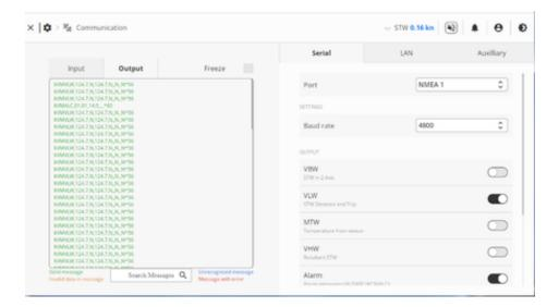
The left side of the display shows a terminal emulator of the information arriving or leaving the system. The user can change from output to input, freeze the screen or filter for a particular message. The colour code of the messages will show their validity.
