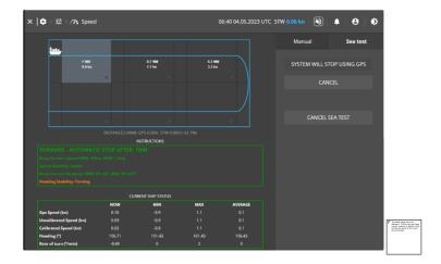
The vessel sails at the same **Heading**, until the correct distance is reached. It will then stop (or be manually stopped by the crew if GPS is not available)
