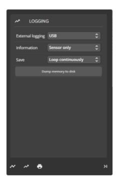
In addition, a USD or microSD disk can be used to log. in this case the old files can be dumped onto the disk, and then new files are written directly.
